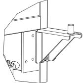
Remove corresponding screws on opposite side of cabinet. On some models there may be a nut behind one or both screws on either side.
