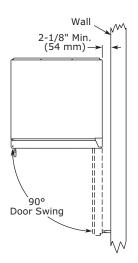
Units have a zero clearance for the door to open 90°, when installed adjacent to cabinets.
