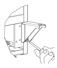
2. Remove corresponding screws on opposite side of cabinet. On some models there may be a nut behind one or both screws on either side.
