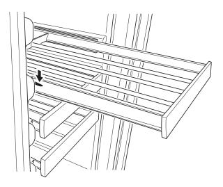
Press the left rack release lever down. At the same time, lift the matching right rack release lever up. Pull the rack out until it is free of the tracks and the cabinet.
