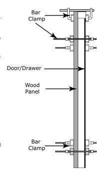
10. Using a 7/64" (3 mm) drill bit, drill 6 pilot holes into the wood panel 1/2" (12 mm)
