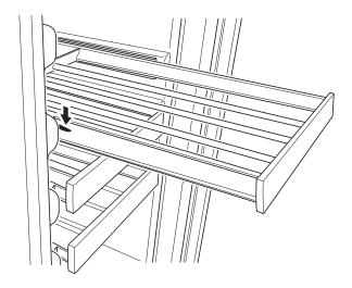
Press the left rack release lever down. At the same time, lift the matching right rack release lever up. Pull the rack out until it is free of the tracks and the cabinet.
