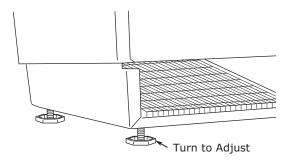
3. Confirm the unit is level after each adjustment and repeat the previous steps until the unit is level.
