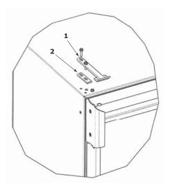
Door latch can be used to prop door open approximately 1/2" (13 mm) when unit is not in use.
