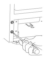
6. Install hinge on opposite side at bottom of cabinet.
