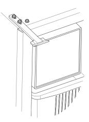
13. Place the door latch assembly on opposite side of unit. Be sure to tighten all three screws securely.
