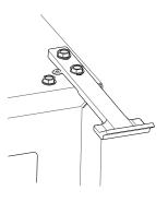
14. Place door on lower hinge pin. Invert and install upper hinge on door. Fasten upper hinge to unit (three screws). Partially tighten screws.
