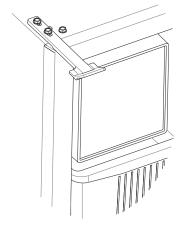
13.Place the door latch assembly on opposite side of unit. Be sure to tighten all three screws securely.
