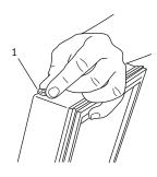
Using a Phillips screwdriver, remove the two screws holding the custom stainless handle from the original location and remove the handle. Remove the two screws on the opposite side of the door. Do not place handle on door until you have completed step 9.
