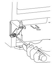
Relocate plastic spacer/bushing on top and bottom of door to opposite side. Clean out bushing hole in door bottom with a screwdriver if necessary.
