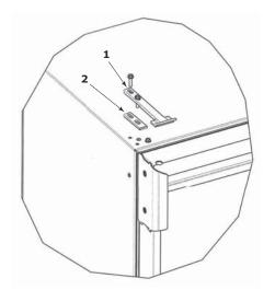
Door latch can be used to prop door open approximately 1/2" (13 mm) when unit is not in use.
